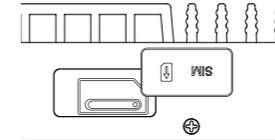
**C** Remove the **SIM tray** with the included SIM Ejector Tool by inserting the tool into the hole on the **SIM tray**; the tray should pop partway out. Remove the SIM tray completely.
