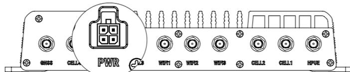
Plug the power cord into the Labeled **PWR** port and a wall outlet
