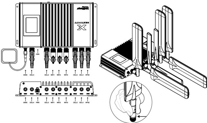
Attach each paddle antenna to its respective port as illustrated by holding the antenna straight and twisting the base to thread onto the connector. Do not overtighten. Finger-tight is sufficient. For optimal signal reception, alternate the antenna orientations as shown above.
