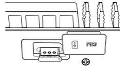
**D** Insert your activated **SIM** into the tray. **Note:** Flip the tray around so that the tray is notched so the card can be inserted the correct way. Press the cover back into place.
