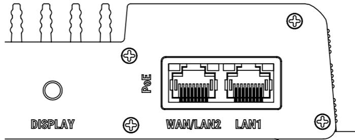
1. Connect your computer to the router **LAN1** port via Ethernet cable or using WiFi with the **SSID** name and password shown on the MegaFi 2 display or from the label underneath the router.
