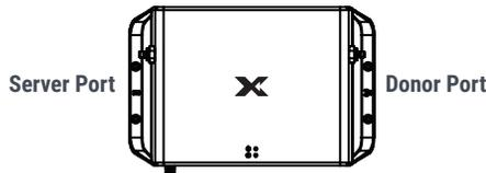
Attach the **Donor Antenna** and **Server Antenna** to the **Main Unit**. Make sure to mount the **Server Antenna** horizontally.
